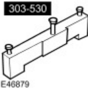
Camshaft setting/locking tool 303-530
